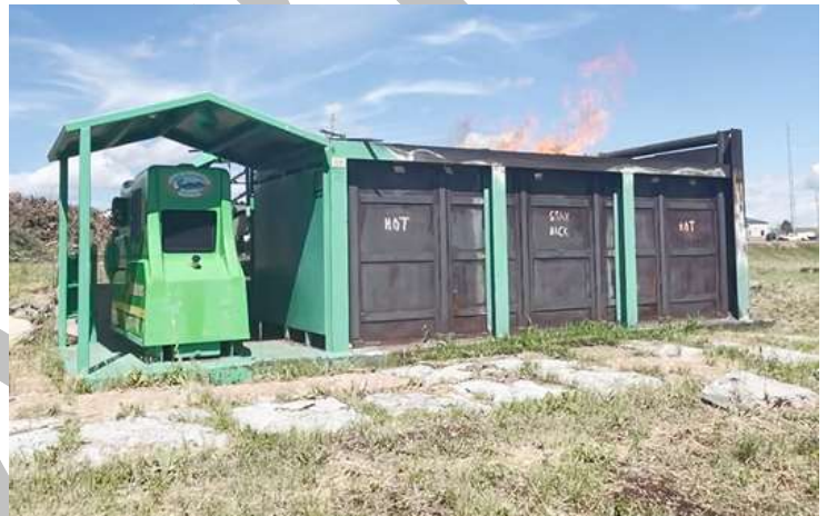
Air curtain burner owned and operated by Loveland Fire Rescue Authority. Photo: TEA
