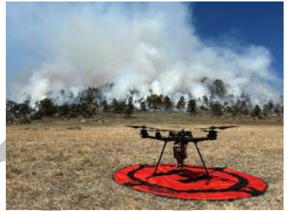
Drones can be used during prescribed burns to determine consumption and effectiveness of interior burning and maintain firefighter safety. Photo from 2023 Magic Feather prescribed burn. Photo credit: USDA Forest Service.
