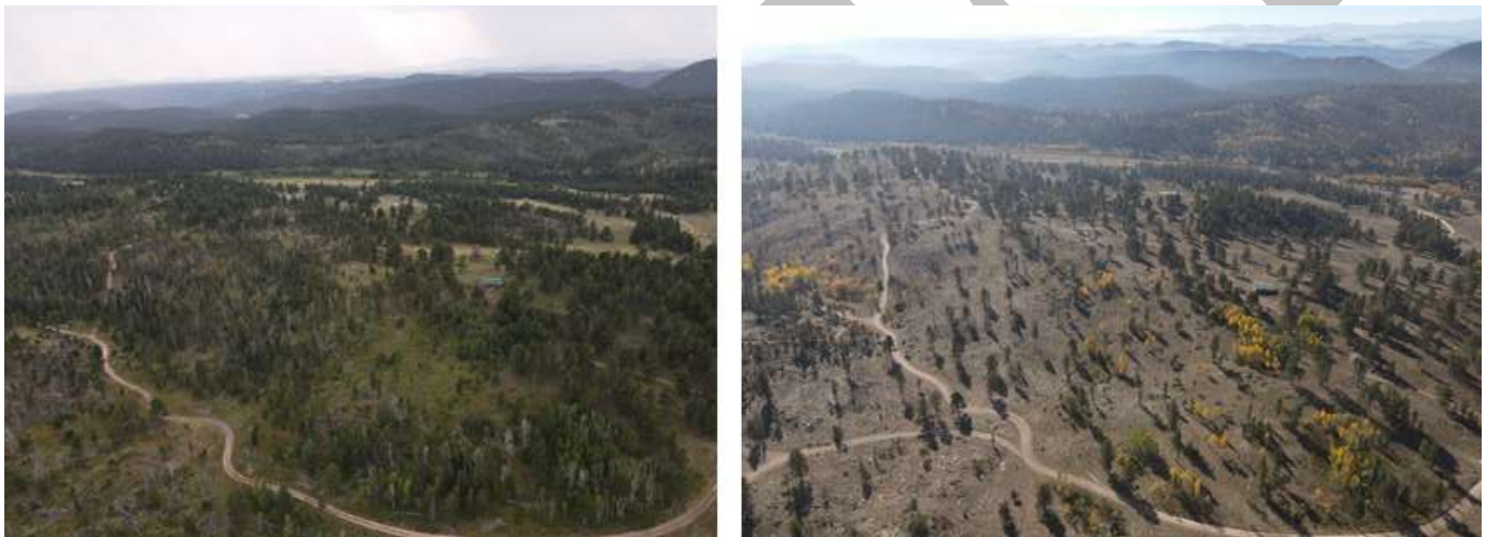
Figure 4.c.1. Before and after aerial imaging of thinning efforts at Poudre River Ranch Road Association. Effective roadway fuel treatments remove enough trees to result in widely space crowns, remove ladder fuels (seedlings, saplings, shrubs, and low limbs), and reduce surface fuels. Removal of trees in large patches mimics the results of fire and reduces ladder and canopy fuel loading to prevent fire from spreading through the canopy. Photo credit: Justin Yow, LCD.
