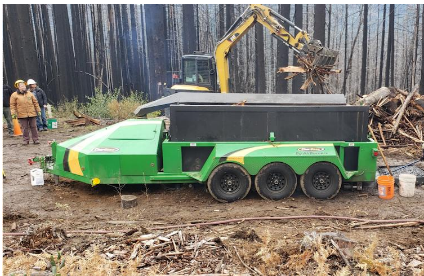
Biochar units can help mitigate wildland fuels and produce biochar that can improve soil health. Photo credit: U.S. Biochar Initiative.
