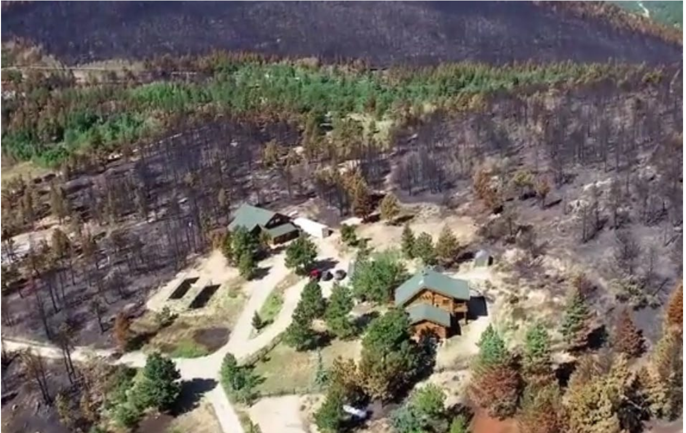
Mitigation in the structure ignition zone allowed firefighters to protect this home during the 2016 Cold Springs Fire near Nederland, CO. Photo credit: Wildfire Partners .
