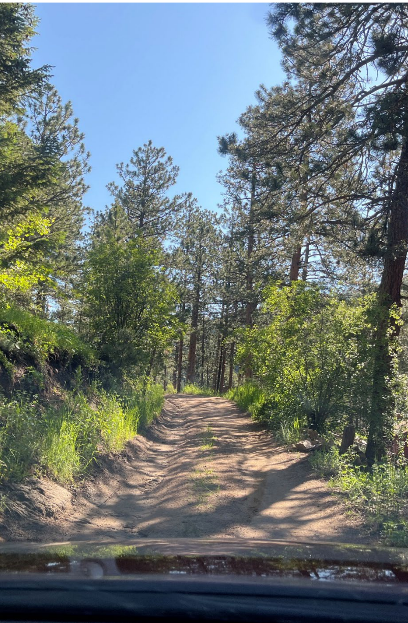
Many driveways within CCCFPD do not meet current access requirements and pose safety issues that are difficult to mitigate. Long, narrow, steep driveways lacking turnarounds, and dense trees on the sides of the road can create challenges for emergency response vehicles during wildfires. Photo credit: The Ember Alliance.
