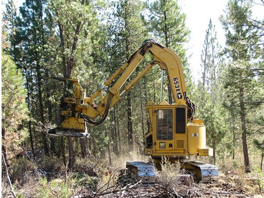
A feller-buncher removes trees in a dense stand of pine trees. This is a common piece of equipment used in mechanical treatment. Photo credit: Oregon Department of Forestry
